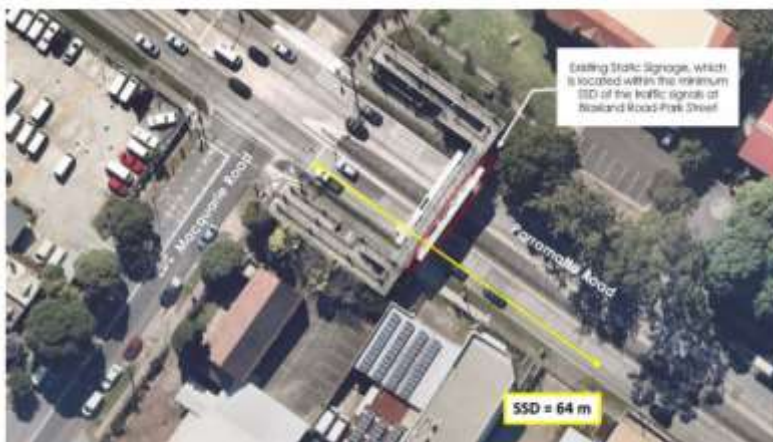
Figure 3-10: Safe Stopping Sight Distance on Parramatta Road
